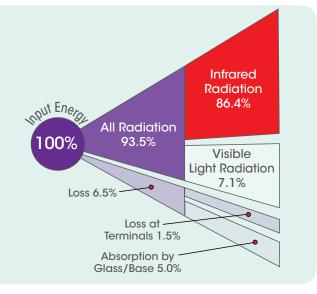
Spectrum Distribution with Fixed Input of Electrical Energy
