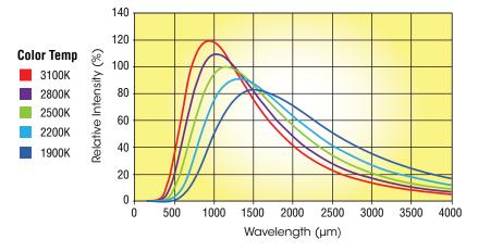
The relative intensity increases as the temperature increases with the resulting peak being shifted towards the shorter wavelength range.
