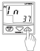
For example, to select thermocouple type E (°F), set the range code to 37.
